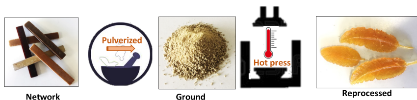
Figure 2. Mechanical reprocessing of ESFO/DTBA thermoset by hot pressing.
