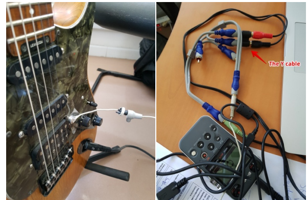
Figure 8: Latency measurement setup
