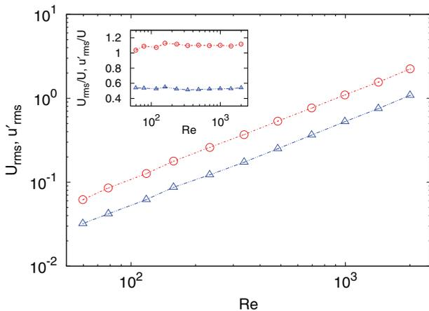
FIG. 1. (Color online) The rms velocity  $U_{\text{rms}}$  (red circles) and turbulent fluctuations velocity  $u'_{\text{rms}}$  (blue triangles) as a function of the Reynolds number  $\text{Re} = UL/\nu$ . The inset shows the two rms velocities normalized by the mean velocity amplitude  $U$ .
