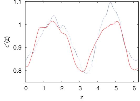
FIG. 4. (Color online) Profiles of local dissipation of the fluctuation energy  $\epsilon'(z) = \overline{\nu (\partial_j u_i')^2}$  normalized with the mean energy input  $FU/2$  for  $Re = 78$  (red solid line) and  $Re = 160$  (blue dotted line).
