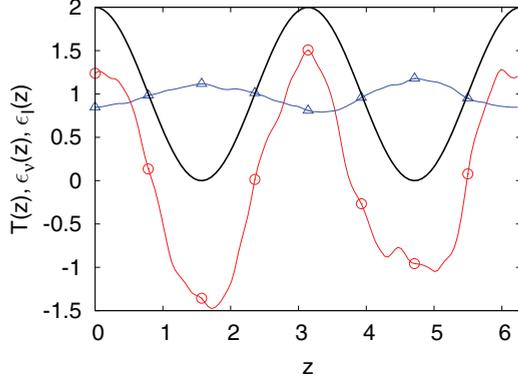
FIG. 3. (Color online) Profiles of energy dissipation  $\epsilon_v(z)$  (blue line with triangles) and energy transport  $T(z)$  (red line with circles), which sum to energy input  $\epsilon_I(z)$  (black line) according to (11). All quantities have been normalized to the mean energy input  $\epsilon_I = FU/2$ . The data are from the simulation at  $Re = 160$ .
